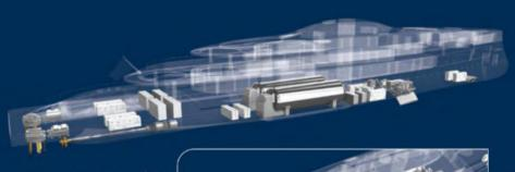
Project Aqua, with an overall length of 112m and 3,530 GT, was developed around a zero-emissions, hydrogenelectric propulsion and energy system. Lateral Naval Architects chose a 28-tonne capacity liquid hydrogen system powering proton-exchangemembrane fuel cells.
