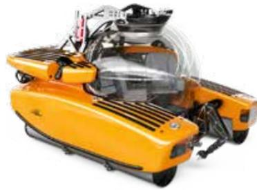
Tried and true, the *Triton 3300/3* is extremely versatile and thus a perfect choice for Esquel. Suited for both personal and scientific expeditions, this sub operates with a pilot and two passengers. It can travel to depths of 1000 meters (3,300 feet) in safety and comfort. It is the ideal vehicle for wreck diving and for viewing the magic of the underwater world. It was aboard a *Triton 3300/3* that man had his first underwater encounter with a giant squid! More adventures await.
